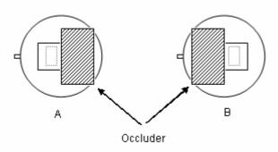
The sensitivity balance of dual elements sensor is calculated by measuring the sensitivity (signal output voltage) of each element and uses the formula as below:
