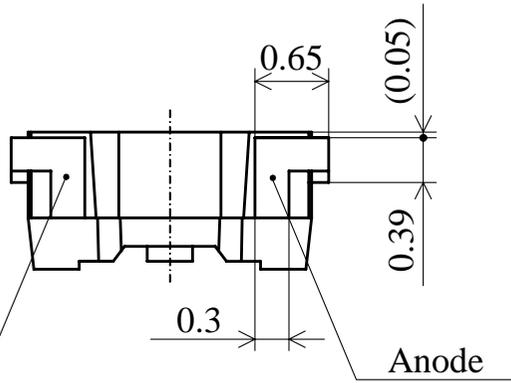
(NOTE) The LED may have flash/flange which exceeds the tolerance of this print.
