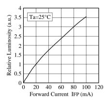
■ Ambient Temperature vs. Relative Luminosity
